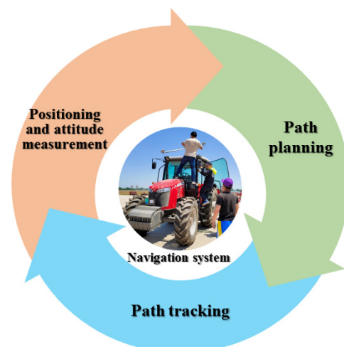
Figure 1. Composition of agricultural machinery automatic navigation system.
