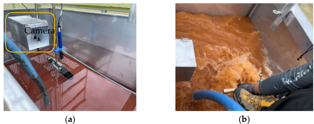
Figure 1. (a) Experimental water tank and measurement devices and (b) mixing after addition of suspended sediment.
