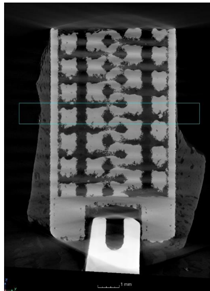
Figure 10. Two-dimensional (2D) XCT sagittal slice of the side-closed implant, open at its bottom, labeled 1386. The blue rectangle is indicating the sections where the BICs were evaluated.
