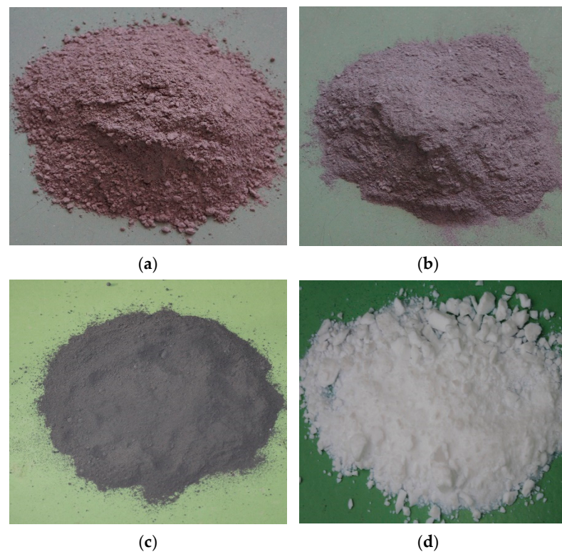
Figure 2. Appearance of binders used: (a) OPC, (b) FA, (c) SF, (d) nS.
