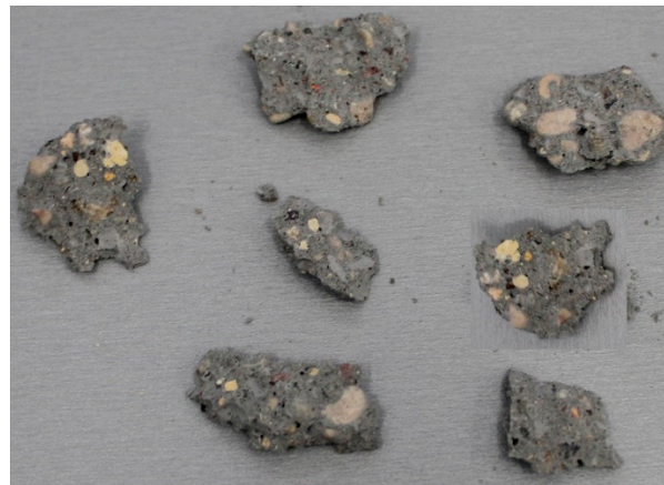
Figure 4. View of samples prepared for SEM tests.
