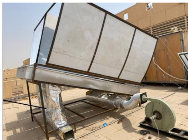
Figure 9. Experimental setup for solar air testing.
