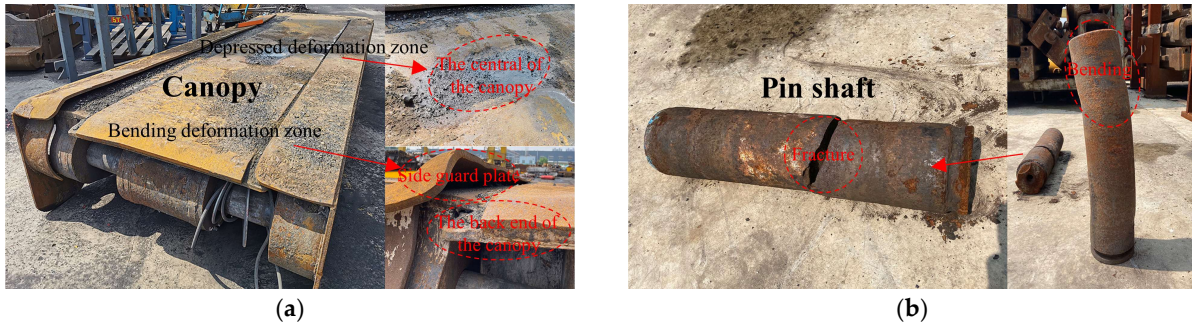
Figure 1. Failure modes of hydraulic support: (a) Failure modes of the canopy, (b) Failure modes of the pin shaft.
