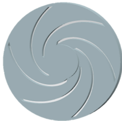
Figure 3. Impeller fluid domain model diagram.
