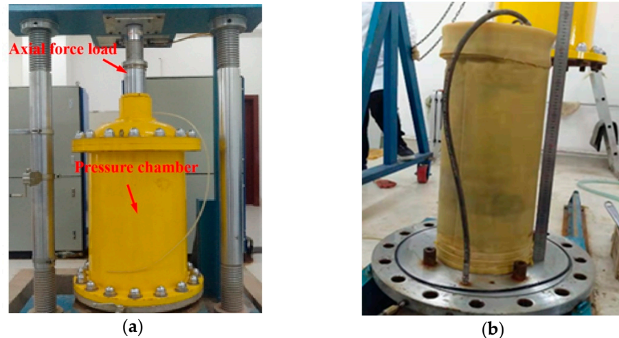
Figure 6. Large-scale SZLB-4 triaxial apparatus and a specimen of the strongly weathered argillaceous sandstone. (a) Triaxial apparatus, (b) Specimen.
