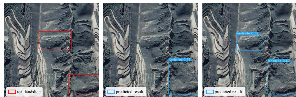
Figure 11. Real landslide and predicted results of the YOLOv5s and LP-YOLO models. (Left) Ground truth box for sparse landslide; (middle) YOLOv5s prediction; (right) LP-YOLO model prediction.
