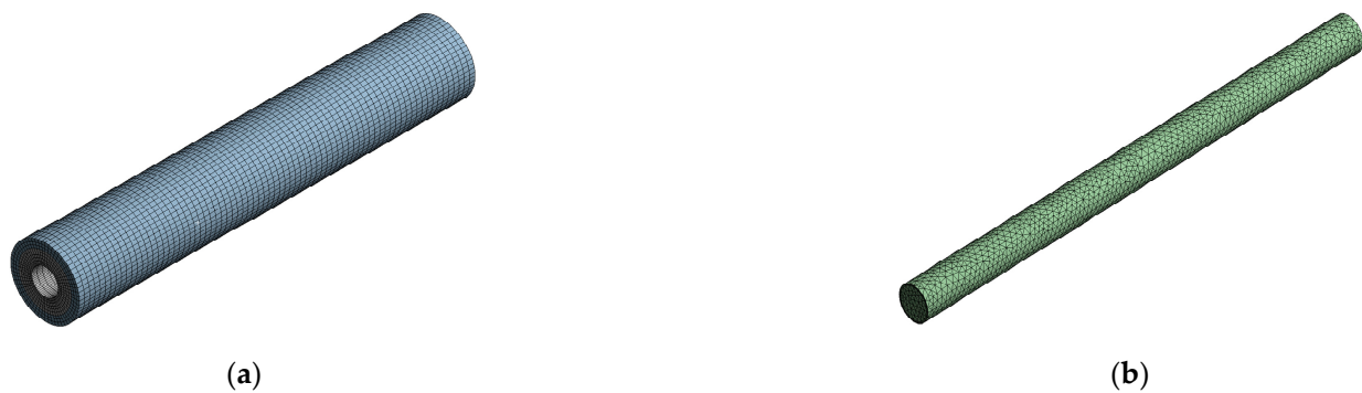
Figure 8. Meshing in the BHP model. (a) Solid region sweep meshing method; (b) fluid region meshing method.
