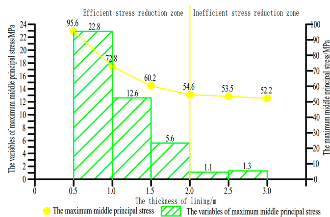
Figure 28. The comparison of the maximum intermediate principal stress under different lining thicknesses.
