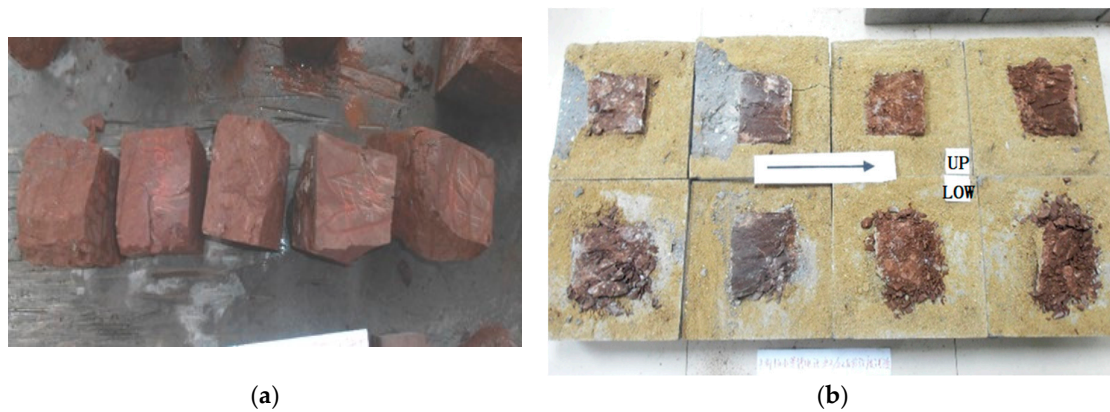
Figure 11. Mudstone post-test sections. (a) Before the test; (b) after the test.
