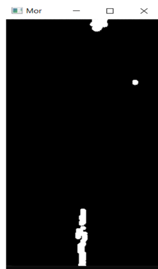
Figure 10. The defect is clearly defined and now stands out as a result of using the morphological operator.
