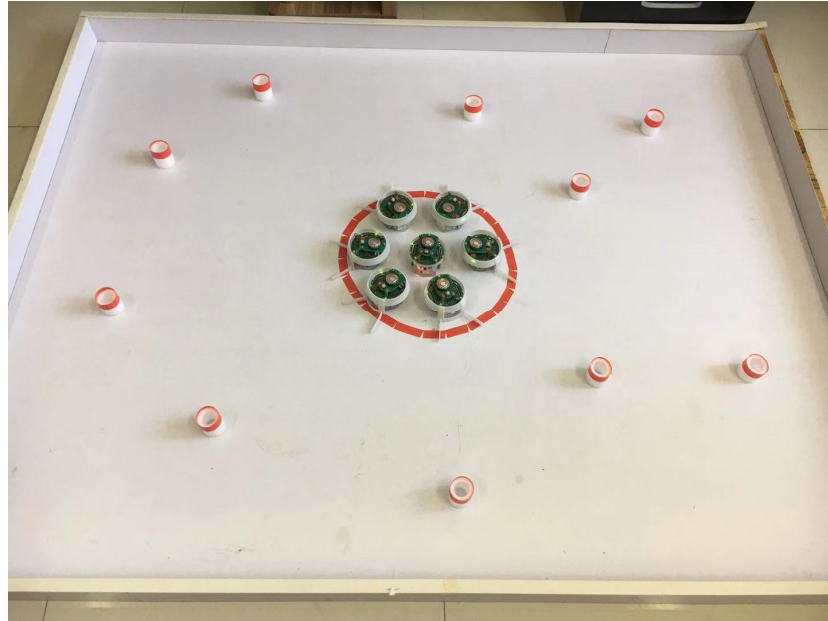
Figure 8. Experimental environment for performing swarm foraging.
