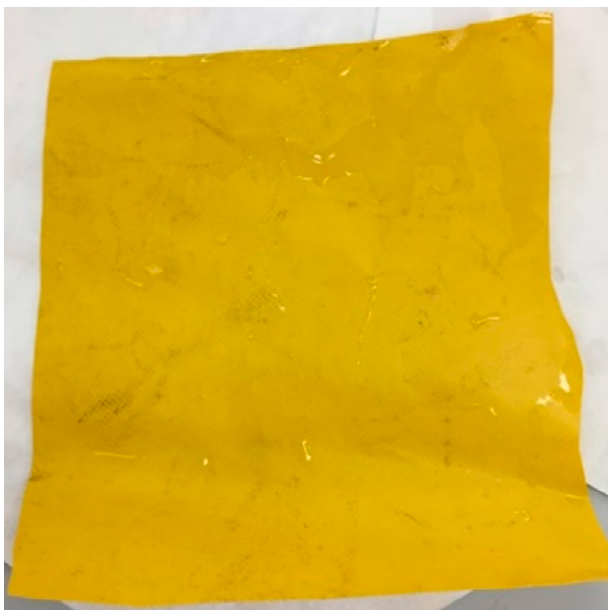
(c) Effect of \text{H}_2\text{O}_2 (hydrogen peroxide) on protective clothing after 60 minutes
