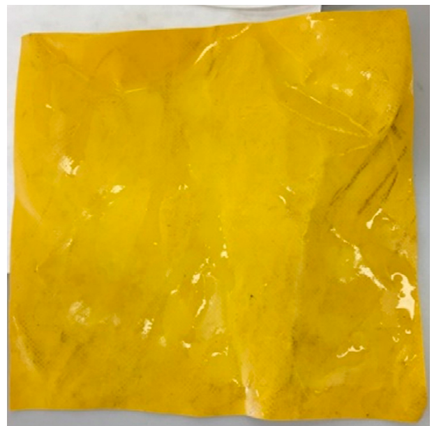
(d) Effect of \text{C}_2\text{H}_6\text{OS} (dimethyl sulfoxide) on protective clothing after 60 minutes
