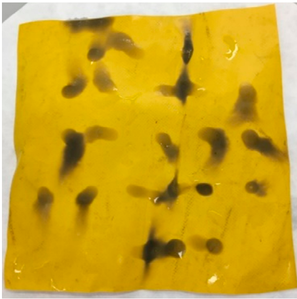
(a) Effect of \text{H}_2\text{SO}_4 (sulfuric acid) on protective clothing after 60 minutes
