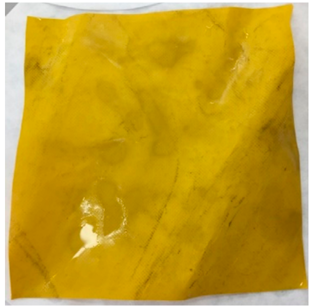
(b) Effect of \text{HNO}_3 (nitric acid) on protective clothing after 60 minutes
