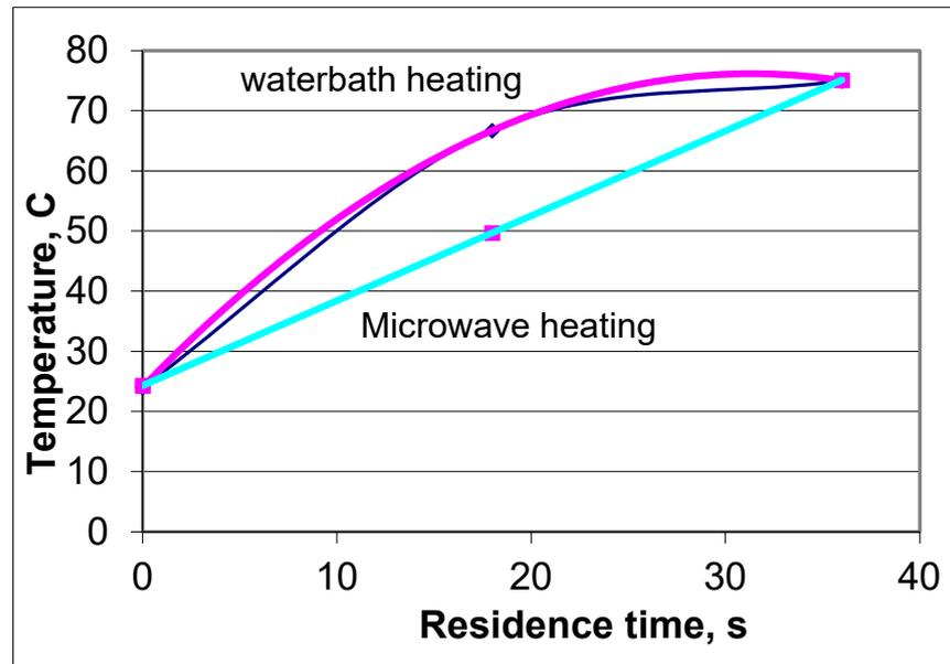
**Figure 8.** Time-temperature profile of the continuous-flow microwave vs. the water-bath heating condition at exit temperature 70 °C. The black and pink lines demonstrate curve fitting.
