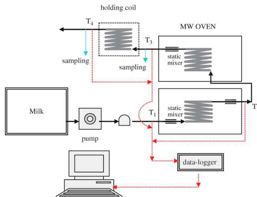
**Figure 1.** Schematics of the microwave heating set-up.
