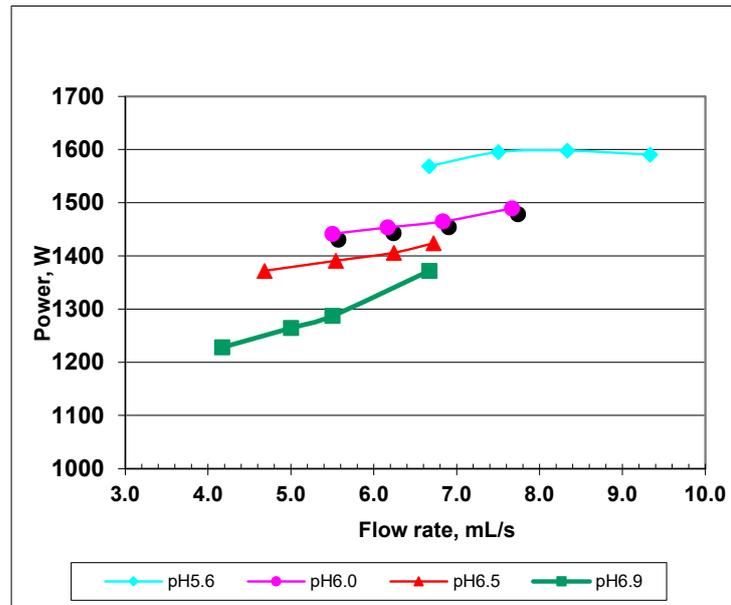
Figure 6. Microwave power absorbed as a function of flow rate at different pH levels.
