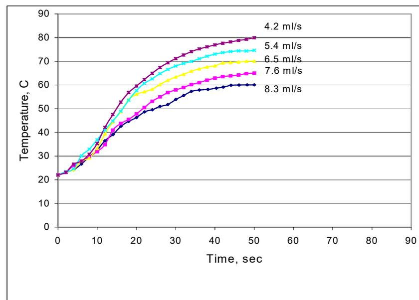
**Figure 2.** Typical microwave heating profiles in the MW system as a function of flow rate.
