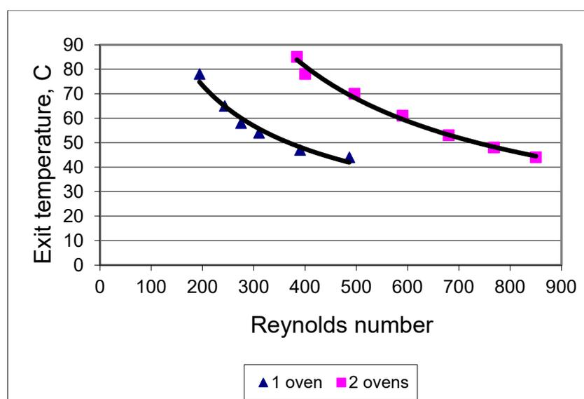
**Figure 5.** Sample temperatures at the microwave exit as a function of Reynolds number.
