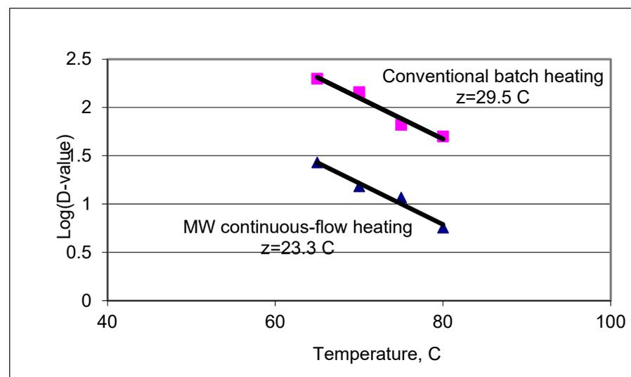
**Figure 9.** Temperature sensitivity comparison between continuous-flow microwave heating and conventional batch heating at pH 5.6.
