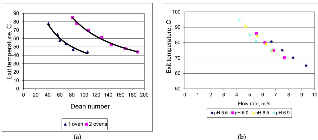
**Figure 4.** Sample temperatures at the microwave exit as a function of (a) Dean number and (b) flow rate.
