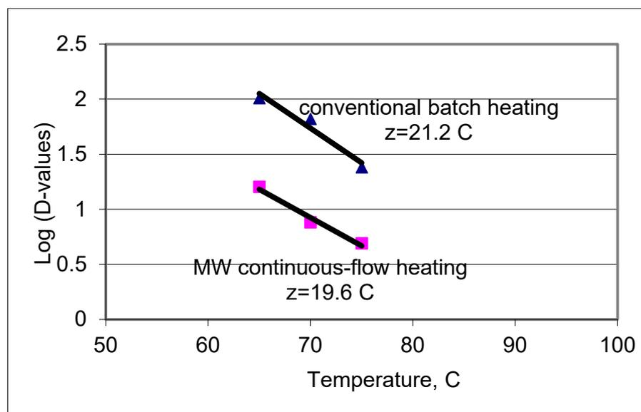
**Figure 10.** Temperature sensitivity comparison between continuous-flow microwave heating and conventional batch heating at pH 5.0.
