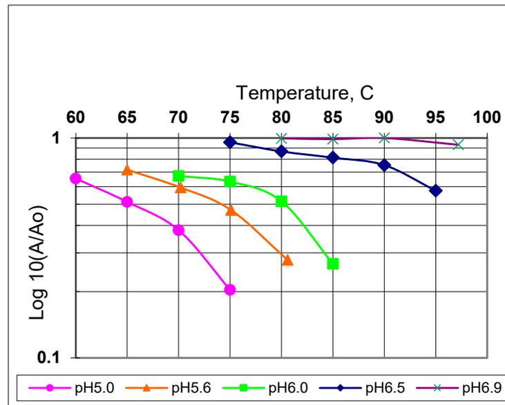
Figure 7. Inactivation rate of TTI from BBA at different pH under continuous-flow microwave condition.
