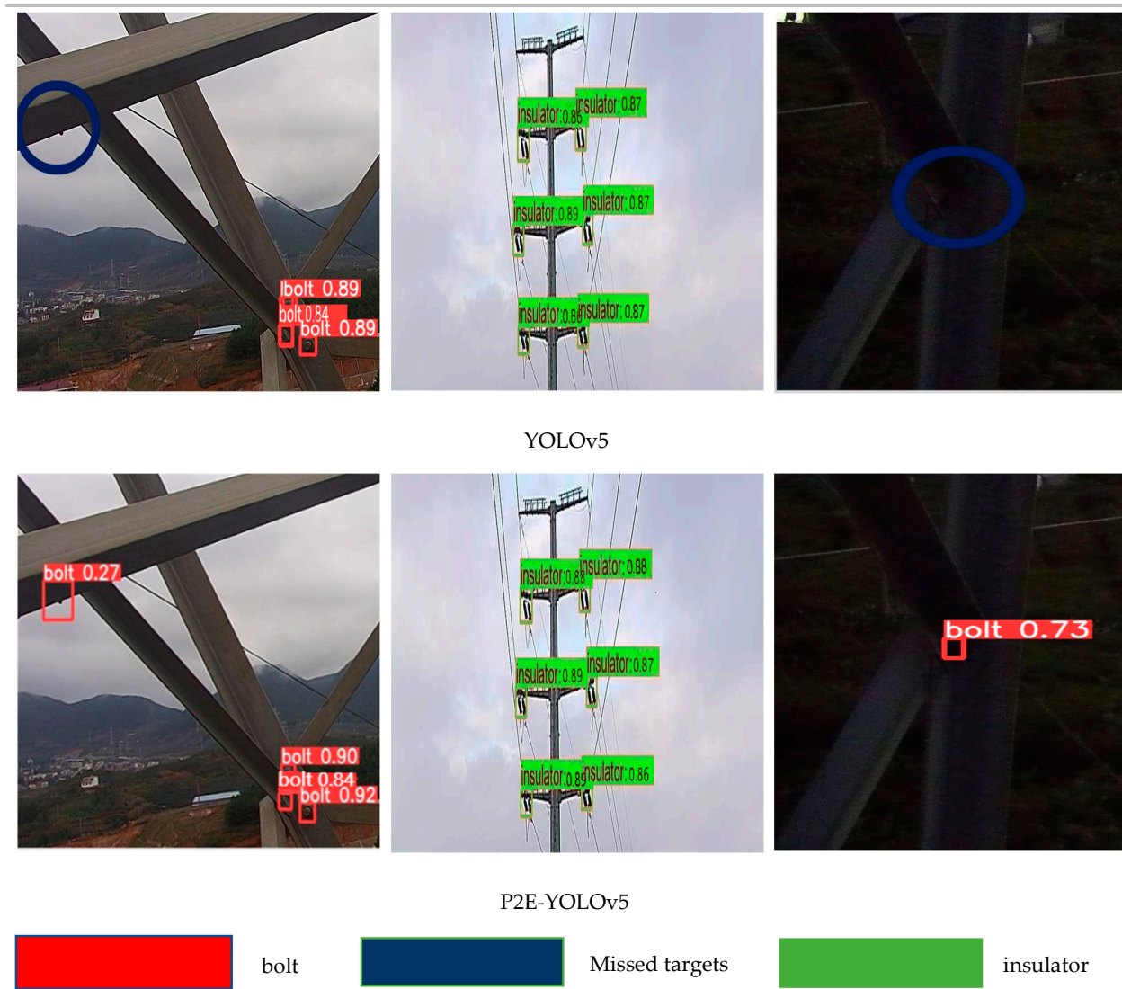
Figure 14. This figure presents a detailed comparison of the detection performance of various algorithms, including Faster-RCNN, RetinaNet, SSD, YOLOv3_spp, YOLOX, YOLOv5, and P2E-YOLOv5, on small targets in transmission line images captured in different scenes.
