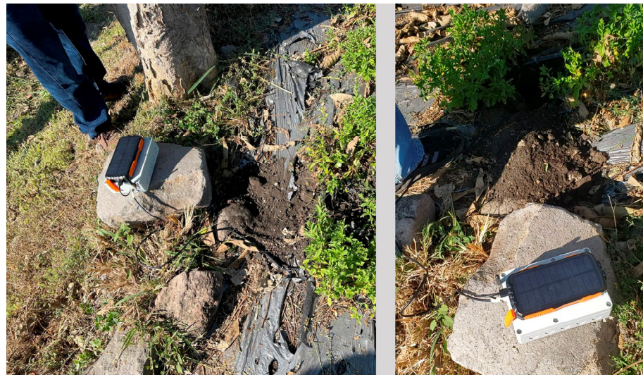
Figure 4. Implementation of a sensor node on a Stevia Morita II crop.
