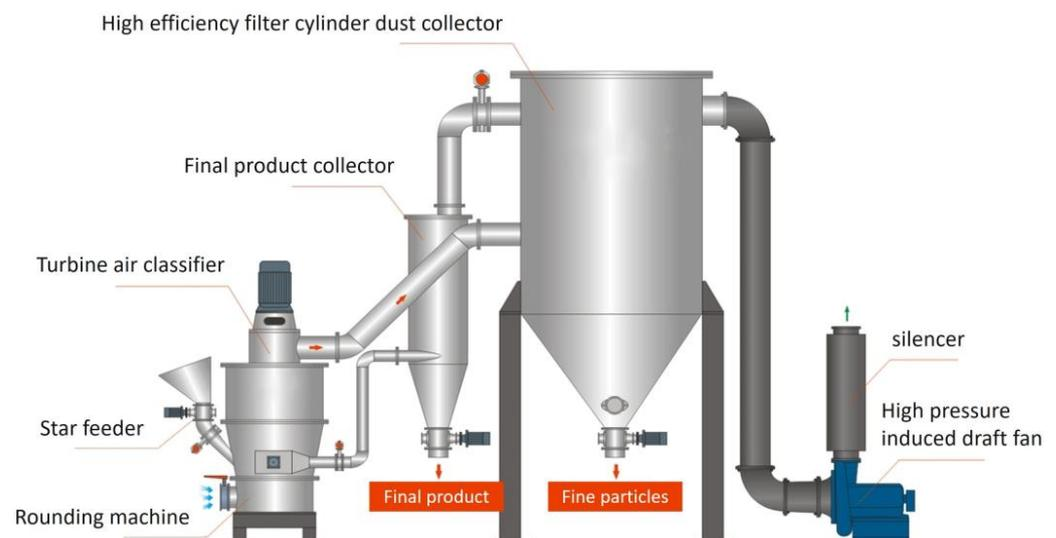
**Figure 3.** Structure of graphite rounding system.
