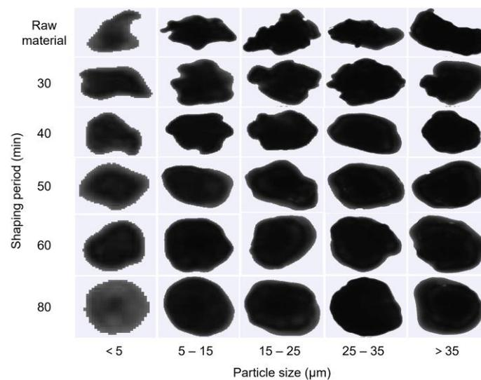
**Figure 8.** The Shape of graphite particles with different size distributions impacted by the shaping period from 30 to 80 min under shaping disk rotating speed at 1833 rpm.
