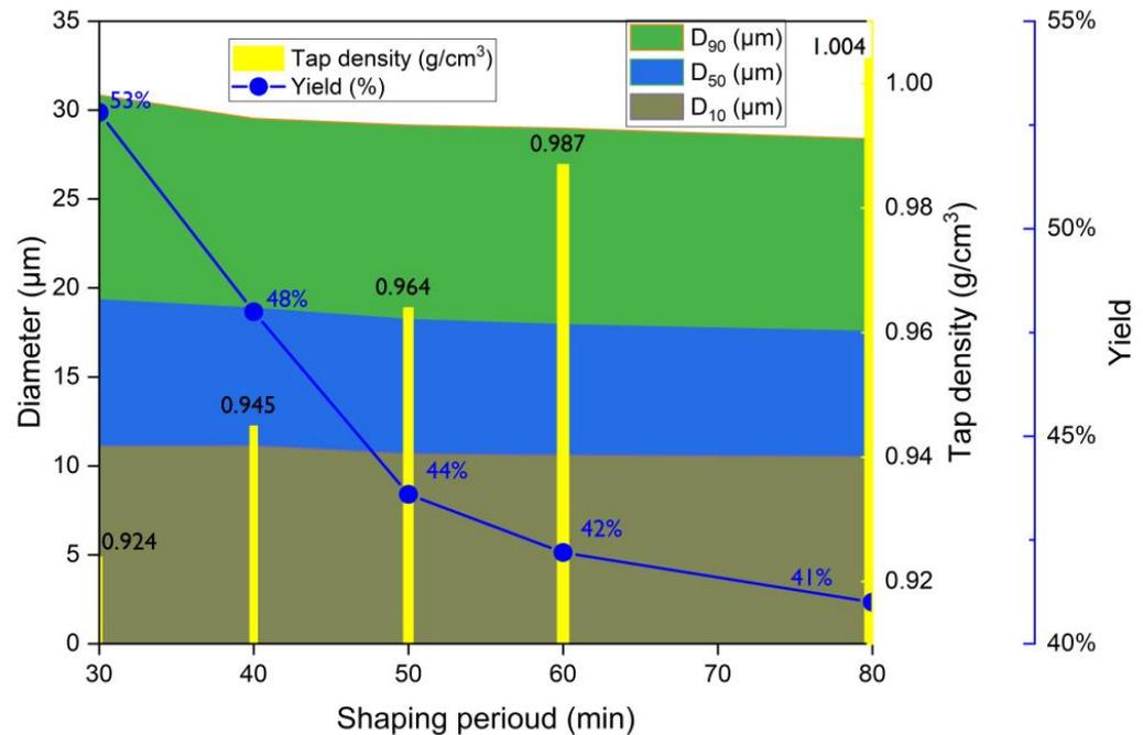
**Figure 5.** Effect of the shaping period on the graphite rounding performance.
