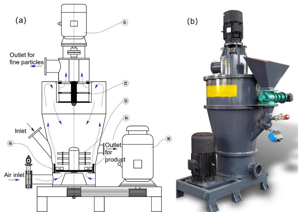
**Figure 2.** Structure (a) and photo (b) of the proposed rounding machine for graphite. (01: classifier motor; 02: turbine rotor; 03: shaping disk; 04: shaping frame; 05: gear ring; 06: shaper motor).
