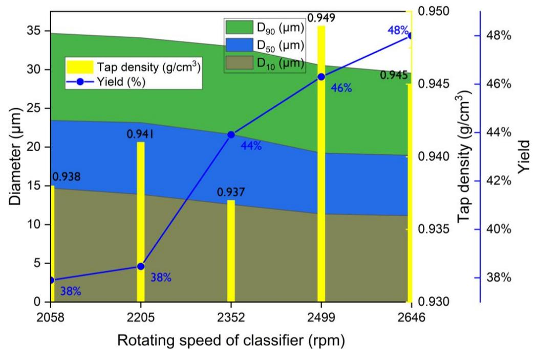
**Figure 6.** Effect of the rotating speed of the classifier on the graphite rounding performance.
