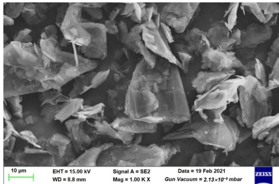
**Figure 1.** Scanning electron microscopy (SEM) of the raw material used in this study.
