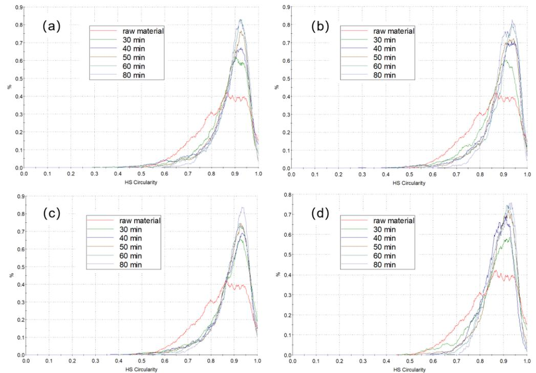
**Figure 7.** Degree of sphericity of graphite particle for different shaping periods at shaping disk rotating speed of (a) 1283, (b) 1467, (c) 1650, and (d) 1833 rpm.
