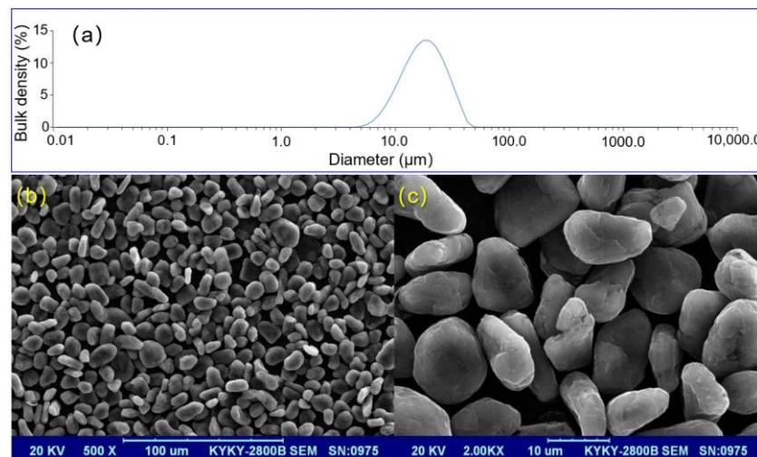
**Figure 9.** Diameter distribution of the final rounding product of graphite (a); scanning electron microscopy (SEM) of the final rounding product of graphite by (b) 500 $\times$  and (c) 2000 $\times$ .
