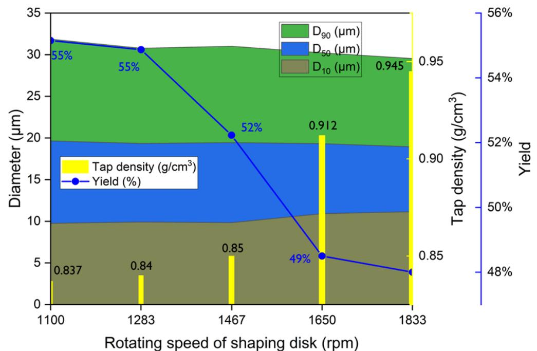
**Figure 4.** Effect of the rotating speed of shaping disk on the graphite rounding performance.
