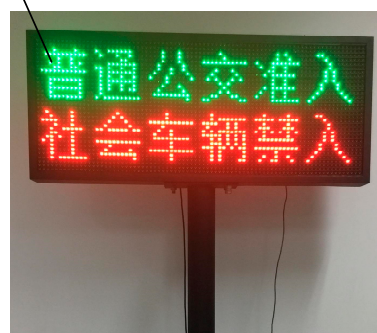
Figure 3. Lane control signals displayed by a VMS.
