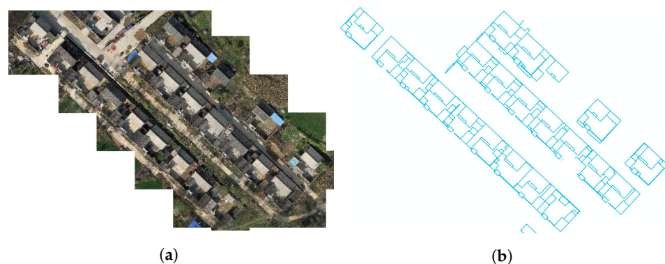
Figure 4. Overall view of the input point cloud and reference vector map. (a) Input color point clouds. (b) Manual reference vector map.
