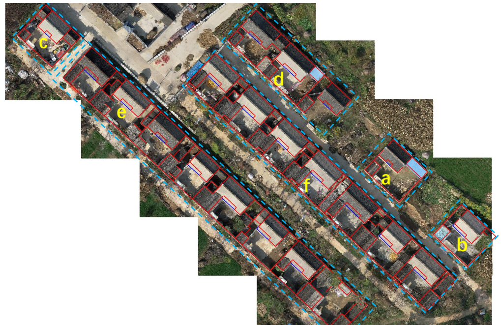
Figure 5. Overall view of the regularized boundaries detected from dense points. Red lines: boundary edges from wall points, and blue lines: extracted doorway boundaries.
