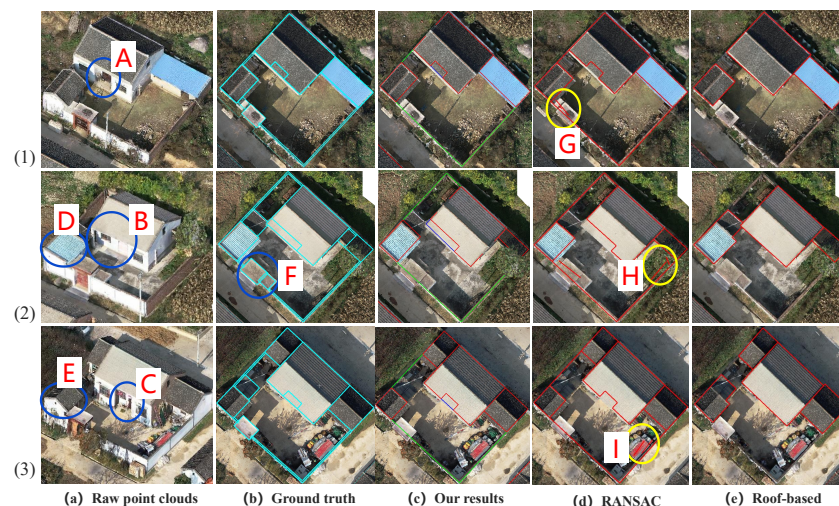
Figure 7. Comparison of local details. From left to right are input point clouds, ground truth, our results, and results of classical RANSAC and direct output from roof point clouds. For areas A, B, and C, incomplete results will be caused by porches for compared methods; for D and E, roof-based approaches are more likely to produce enlarged boundaries; for G, H, and I, spurious lines are extracted for traditional RANSAC-based methods.
