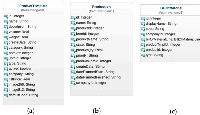
Figure 19. (a) ProductTemplate class; (b) Production class; (c) BillOfMaterial class.
