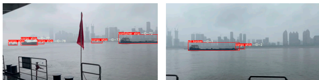
Figure 10. Cargo ship and oil tanker tracking in poor visibility.
