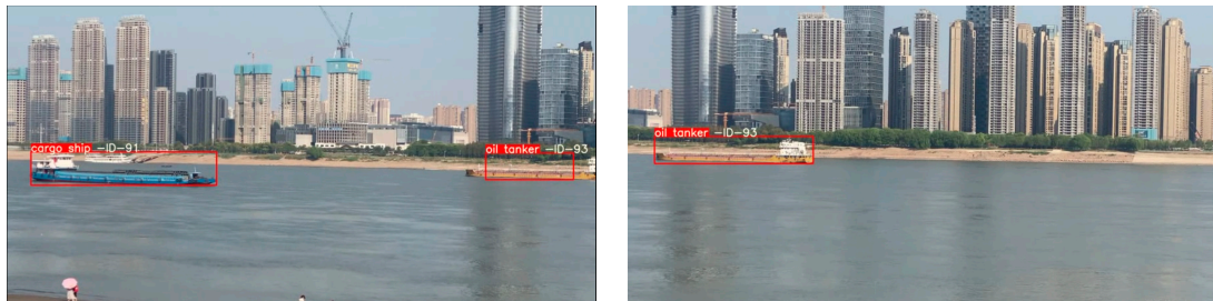
Figure 8. Cargo ship and oil tanker tracking in good visibility.
