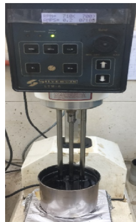
Figure 2. The high-shear mixer for blending the modified asphalt binders.
