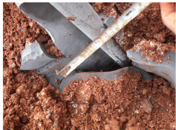
(b) splitting channel of the cement slurry.
