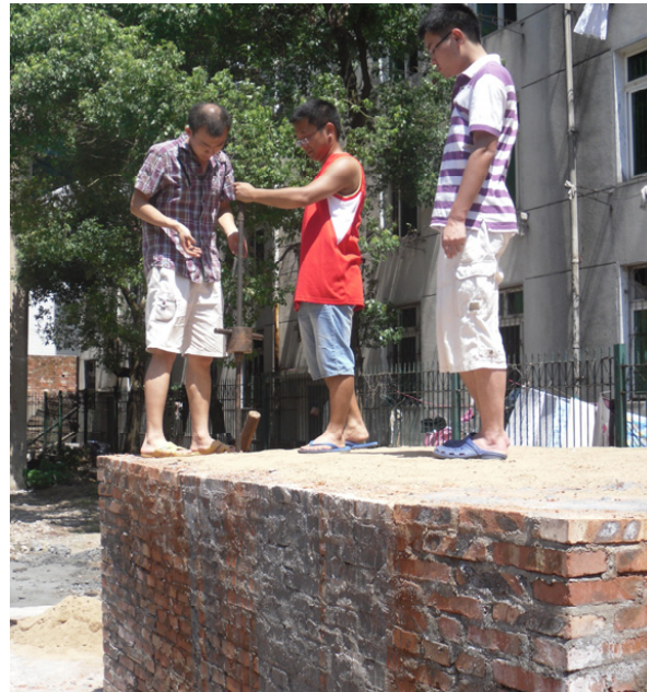
Figure 12. Field light dynamic penetration test.
