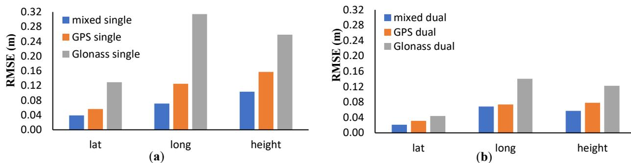
**Figure 6.** Kinematic PPP RMSE from GPS, GLONASS, and mixed GPS/GLONASS using (a) single-frequency observations, and (b) dual-frequency observations.
