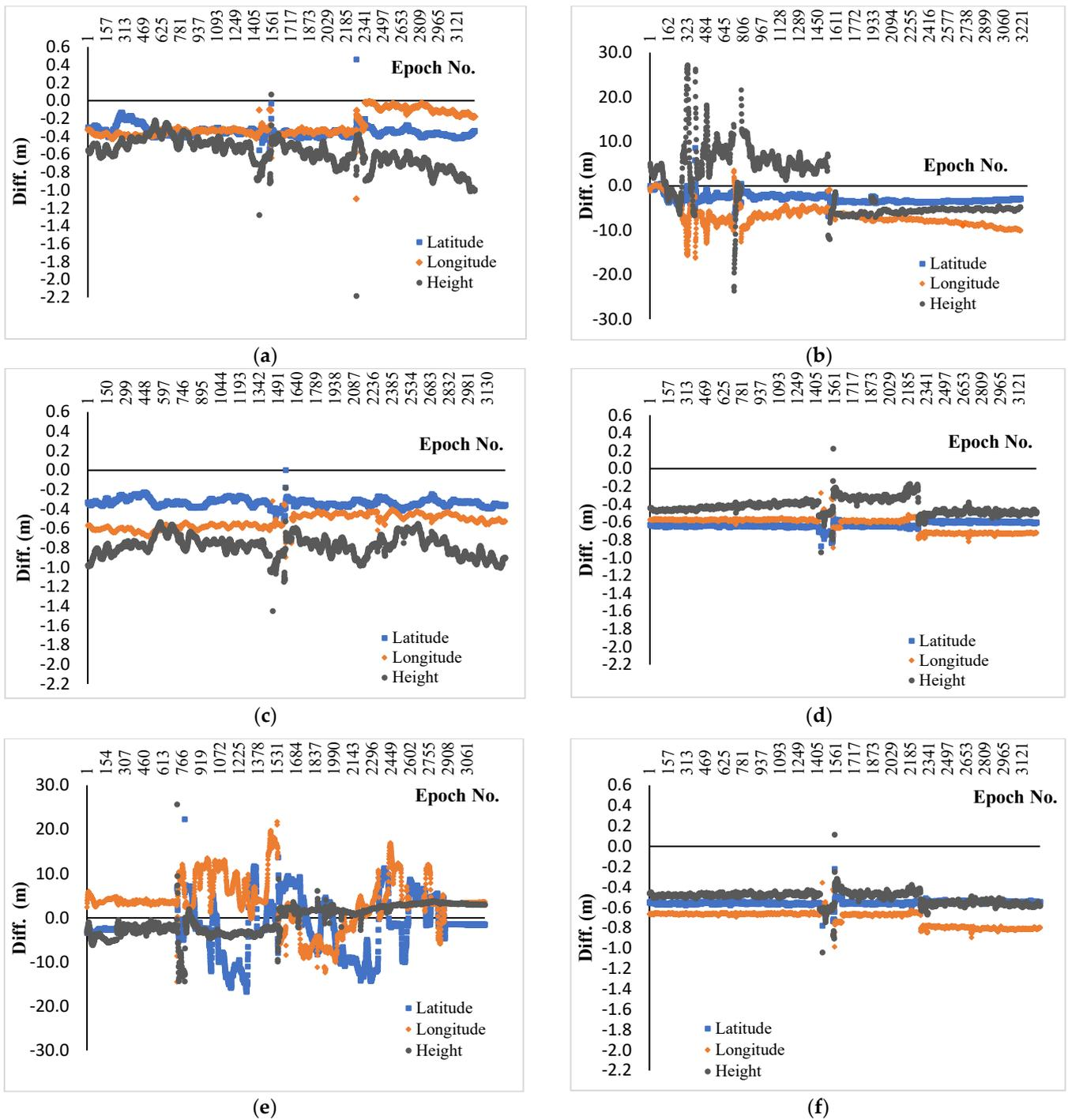
**Figure 5.** Kinematic PPP coordinate differences using (a) GPS single-frequency observations, (b) GLONASS single-frequency observations, (c) mixed GPS/GLONASS single-frequency observations, (d) GPS dual-frequency observations, (e) GLONASS dual-frequency observations, and (f) mixed GPS/GLONASS dual-frequency observations.
