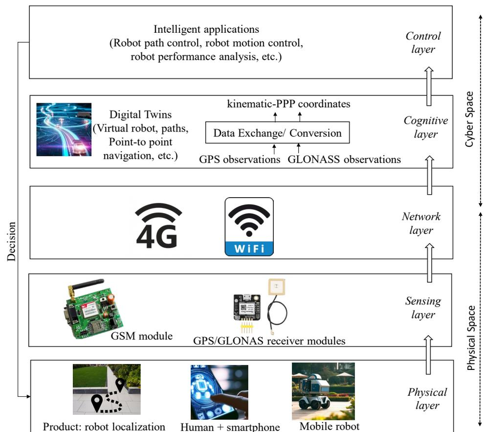
Figure 1. The architecture of CPS-based mobile robots for localization function.
