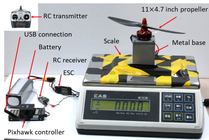
Figure 14. Experiment to find out the relationships between PWM (to ESC) and the rotor thrust.
