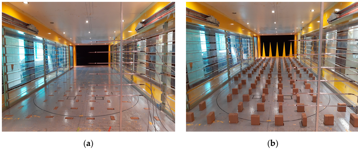
Figure 8. The view of the aerodynamic tunnel for (a) “quasi-laminar” flow and (b) turbulent flow. On the left side, there is a vertical rod with six thermo-anemometers for wind profile estimation.
