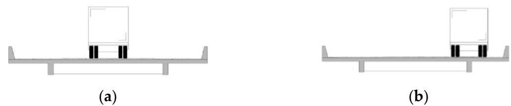
Figure 4. Passage of the three-axle rigid vehicle [3C]. (a) Along the center line of the bridge. (b) Over the right girder (G1).
