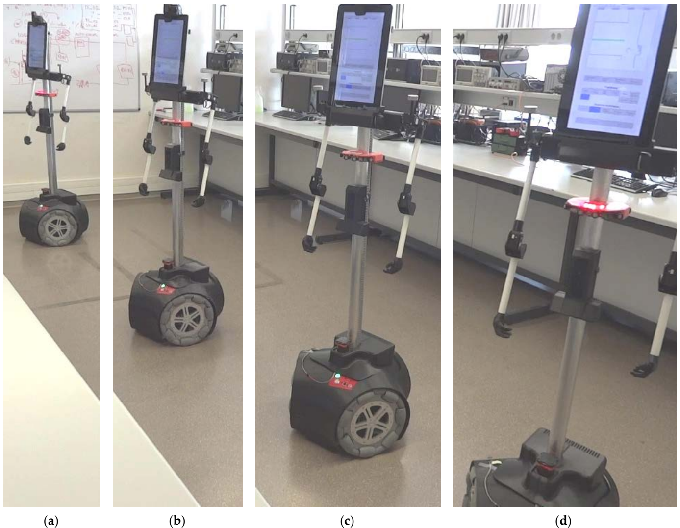
Figure 1. APR-02 mobile robot performing a transversal (or lateral) displacement: (a) starting point; (b,c) intermediate points; and (d) destination point.
