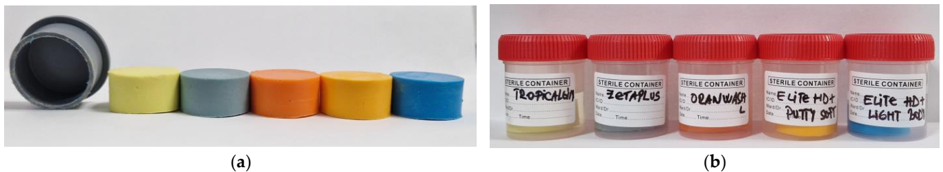
Figure 2. Preparation of the specimens: (a) the plastic plug and one specimen from each impression material; (b) the containers with the microorganisms and the specimens.
