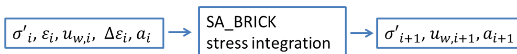
Figure 6. Scheme of the SA_BRICK stress integration procedure in the form of the PLAXIS user-defined soil model.
