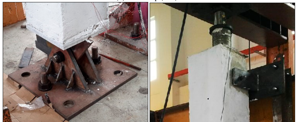
(c) Hinge supports at the joint.
