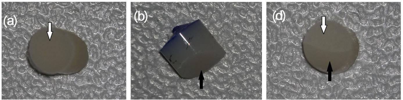
**Figure 2.** Representative optical microscope images (15× magnification) for each category of failure mode observed in the study. (a) Adhesive; (b) Cohesive in resin bulk; and (c) Mixed. White arrows indicate the adhesive agent and black arrows the resin cement.
