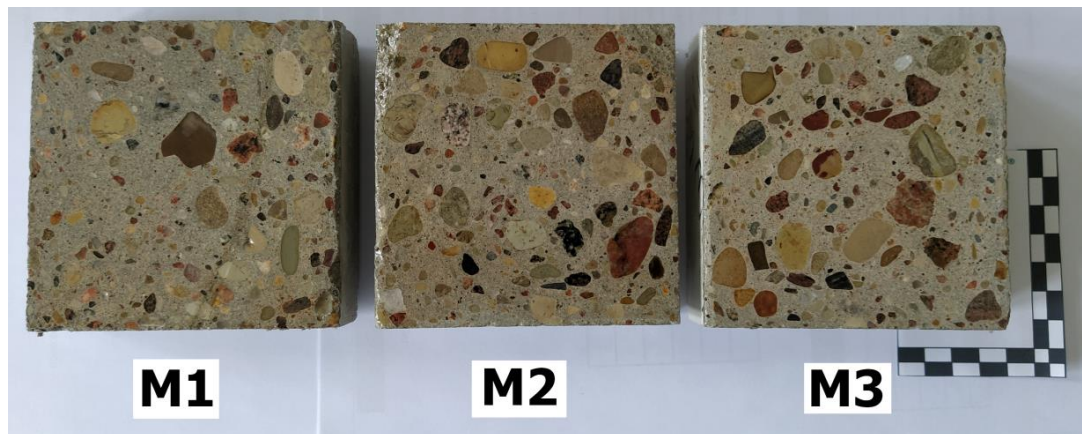
Figure 4. Pre-polished surfaces of concrete samples.
