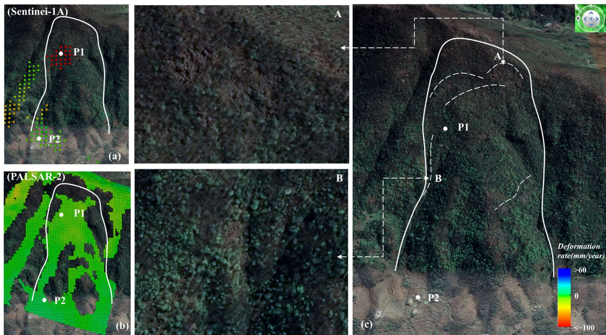
Figure 11. Sanxingwan landslide. (a,b) show annual deformation rate results of ALOS/PALSAR–2 and Sentinel–1A, respectively. (c) is the optical image on Google Earth. The P1 and P2 points marked on the figure are the points for time series deformation analysis in Chapter 5.4.3
