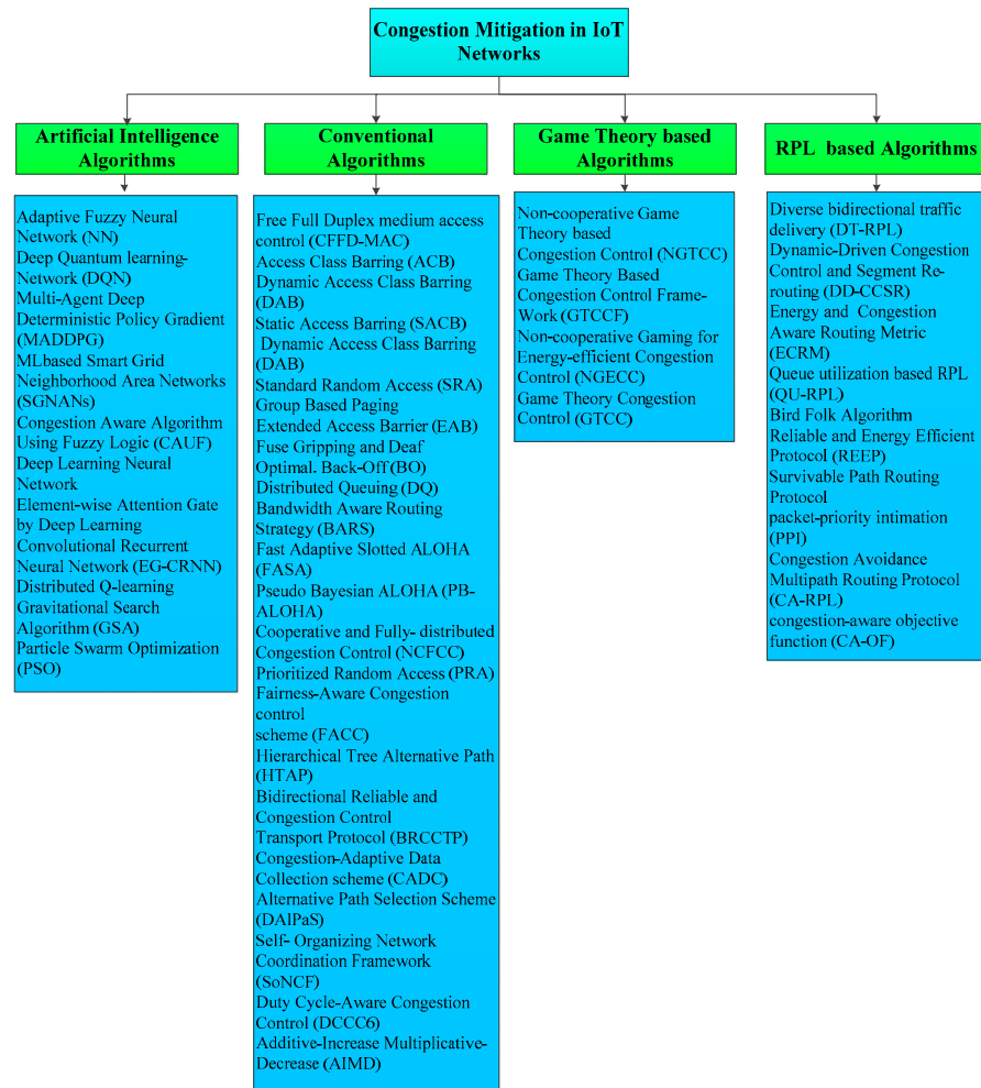
Figure 2. An overview of congestion mitigation AI algorithms in the literature for WSN.
