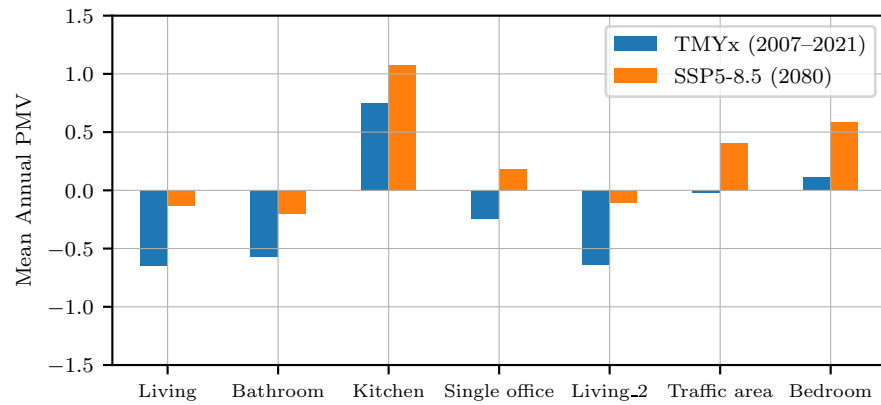
Figure 9. Mean annual PMV per thermal zone comparing the scenarios for TMYx (2007–2021) and SSP5-8.5 (2080) weather data.
