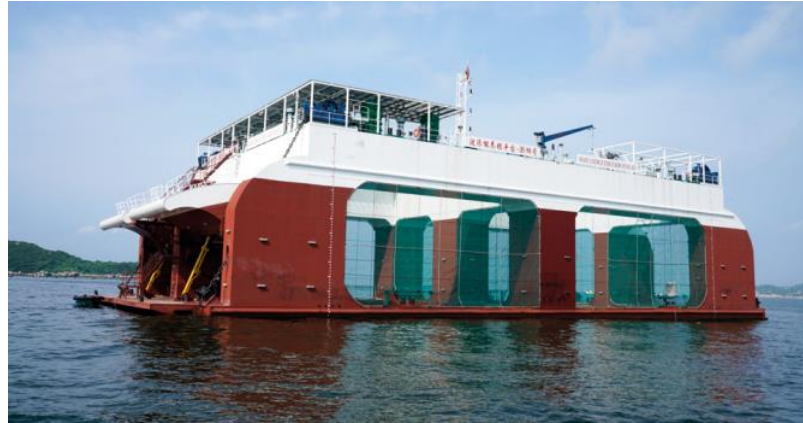
Figure 1. An overview of the semi-submersible aquaculture platform “Penghu” [37].
