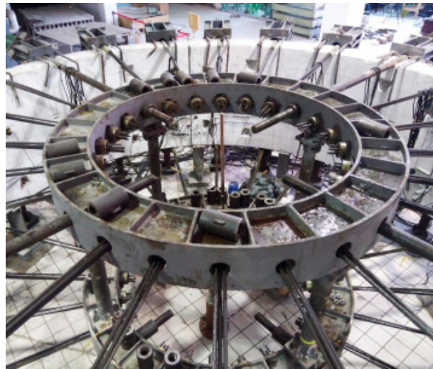
Figure 8. Full-scale model test of shield segment in the literature [24].
