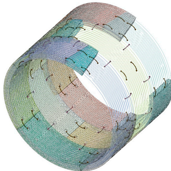
Figure 7. Schematic diagram of the finite-element model of the shield tunnel.
