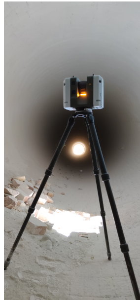
Figure 4. Leica RTC360 inside the rotary kiln.
