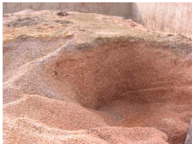
Figure 2. Cargo condensation at the stow peripheries.
