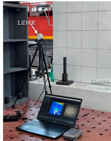
**Figure 6.** An example of non-contact measurement of displacement using LiDAR.
