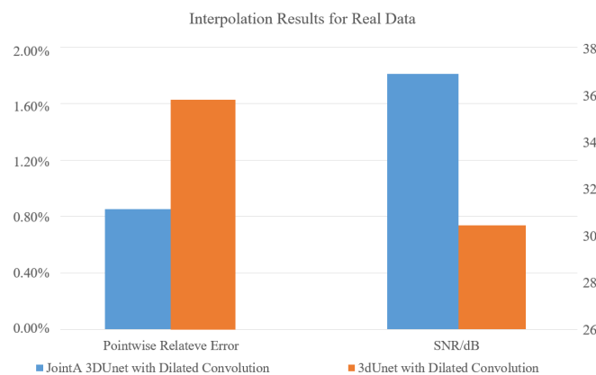
Figure 10. Comparison of interpolation results for real data between 3DUnet and JointA 3DUnet.
