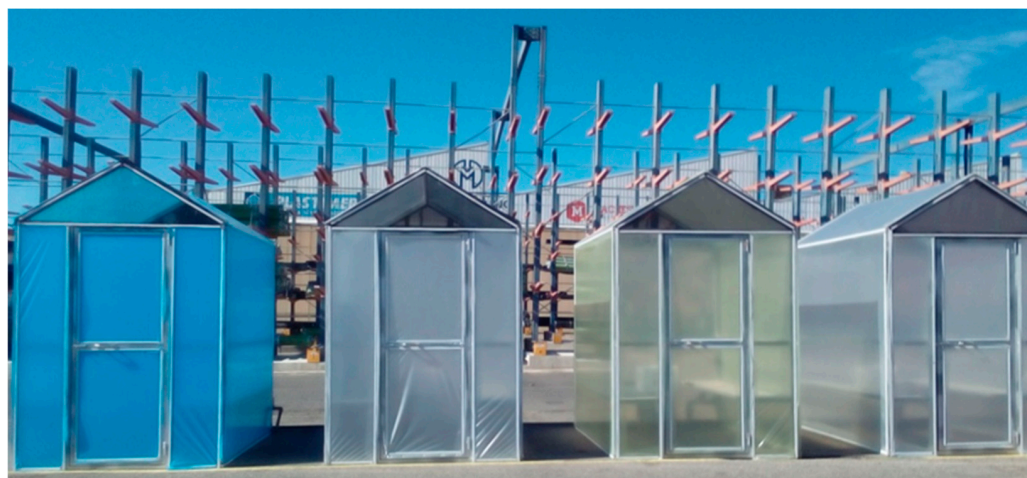
Figure 1. Pilot greenhouses with different covers from left to right blue, grey, yellow and colorless EPCs.
