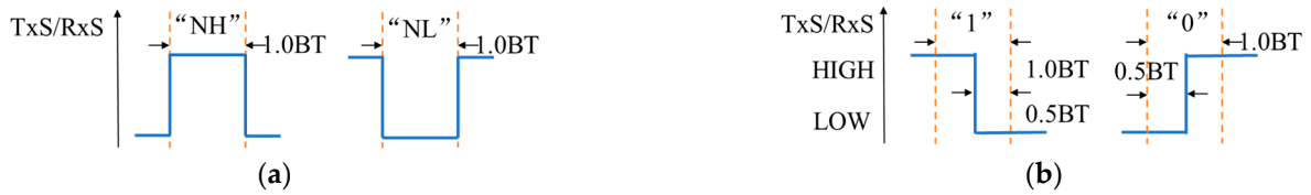
Figure 2. The encoding format of data and non-data symbols: (a) non-data symbol encoding; (b) "0" and "1" data encoding.
