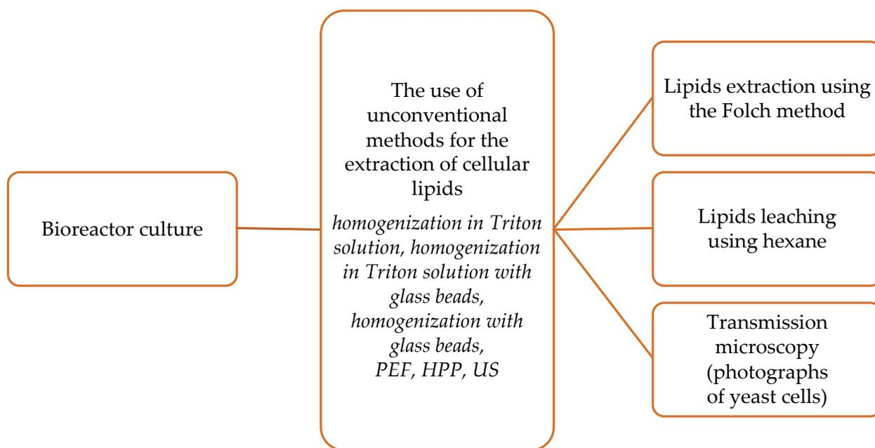
**Figure 2.** Experimental diagram for yeast biomass pretreatment and oil extraction from previously treated yeast cells.
