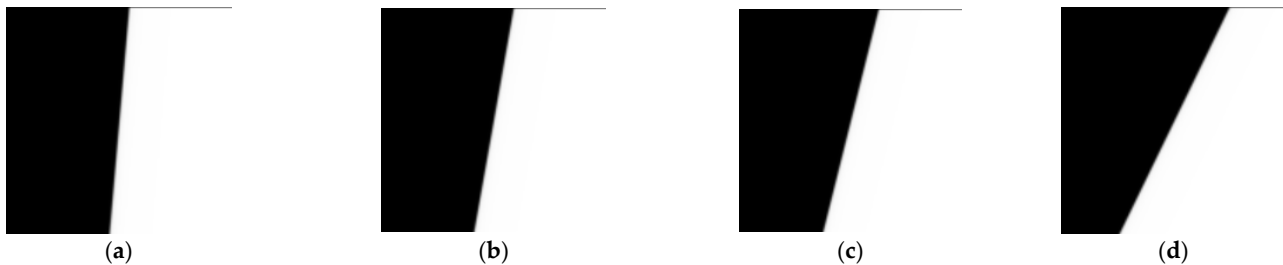
Figure 9. Images of slanted edge with different angles: (a) slanted-edge angle of 5^\circ ; (b) slanted-edge angle of 10^\circ ; (c) slanted-edge angle of 14^\circ ; (d) slanted-edge angle of 26^\circ .
