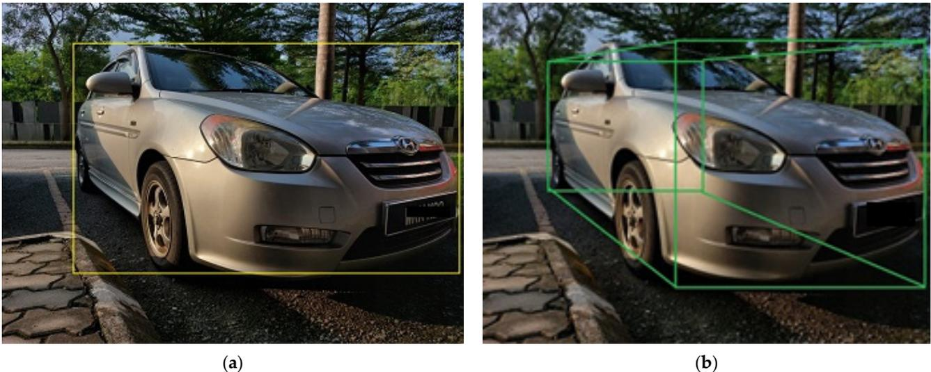
**Figure 1.** (a) Two-dimensional detection of a car; (b) 3D detection of a car.
