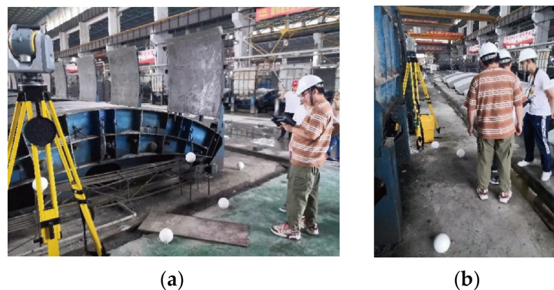
Figure 1. Scanning being performed at a tunnel segment factory in the Panyu District, Guangzhou, China: (a) scanning of a mold for the segment production; (b) scanning of the segment.
