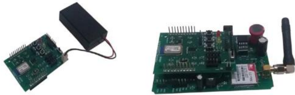
Figure 6. WiSeN sensor node.
